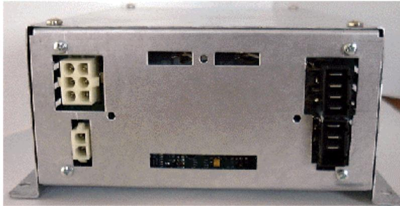
Figure 1 "Prototype version of Mod. AL 310X power supply unit"
