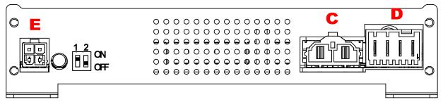
Connector C is the output of the battery to be charged.
