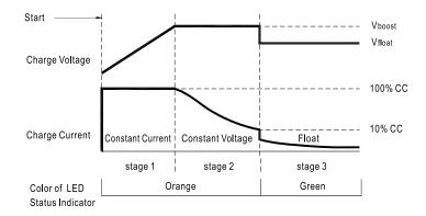
When the DCC is turned on in charging mode, it will maintain a constant current until the battery voltage reaches the Absorption Voltage. The current during this stage may vary throughout operation in order to maintain a safe operating temperature, or to limit the difference between input and output voltages.
