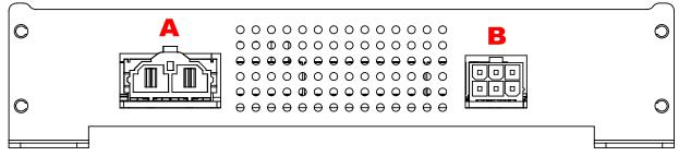
Connector A is the input of the power line from the alternator.
